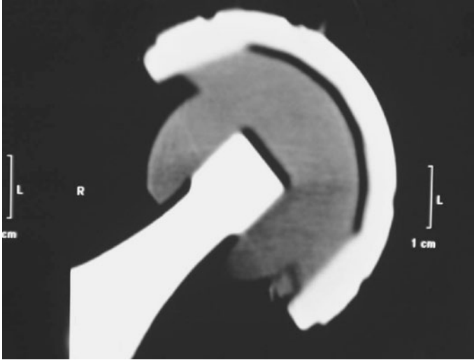
■ Fig. 5 Coronal computer tomogram of the ceramic insert in case 2 showing rim fracture.
