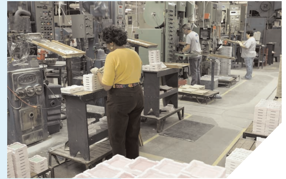
Dry pressing of high volume ceramic insulators.
