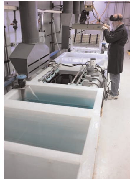
Electrolytic nickel plating of metallized ceramic insulators and other metal components.
