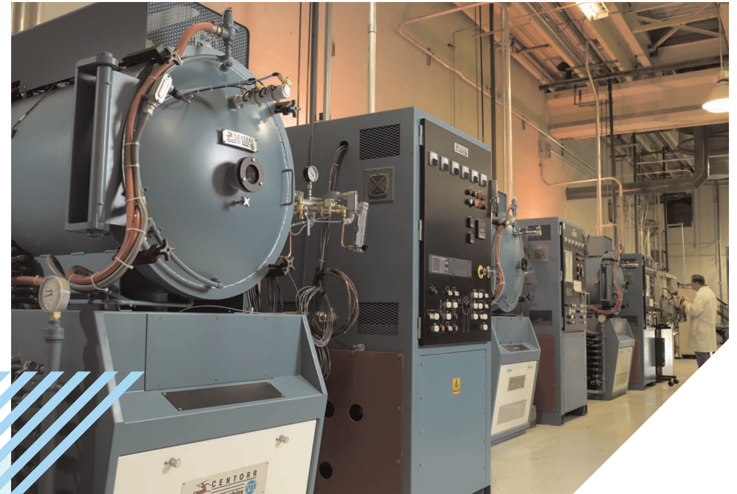
Vacuum brazing furnaces with computer programmed profiles.
